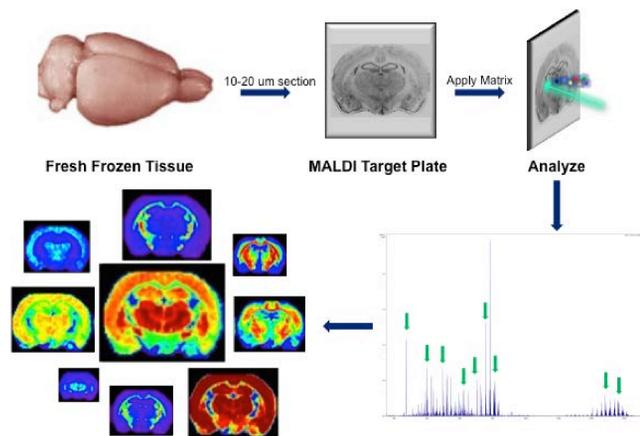
An imaging MALDI MS experiment requires a laser to be systematically rastered across an entire tissue section while acquiring a mass spectrum at each ablation spot. The precise x,y coordinates of the recorded mass spectra are then compiled to represent individual “pixels” in an ion image. Specific m/z values can be selected to produce 2D ion density maps representing the location and relative abundance of an analyte within the tissue sample.
