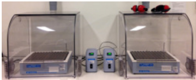
Fig. 4. 2x DigiPREP for digestion of 216 samples (tissue, feces or bone) per run using nitric acid, hydrogen peroxide and controlled heating.
