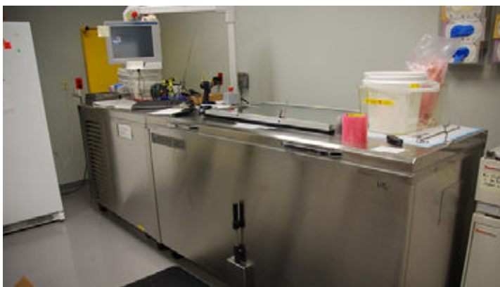
Figure 3. A typical cryomacrotome, used for sectioning animals in QWBA.
