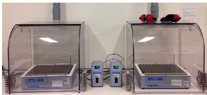
Figure 4: 2x DigiPREP for digestion of 216 samples (tissue, feces or bone) per run using nitric acid, hydrogen peroxide and controlled heating.
